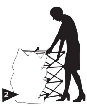
2 Ensure "adjustable feet" of frame are on the floor. Pull up display into upright position.
