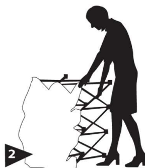
2 Ensure "adjustable feet" of frame are on the floor. Pull up display into upright position.
