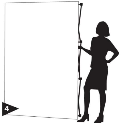
4 Adjust leveling feet for desired angle. Ready pop display can now easily be moved into position.
